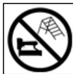
According to the European Norm EN 792-13 the regulation is valid from 01.01.2001 that all fastener driving tools with contact actuation must be marked with the symbol "Do not use on scaffoldings, ladders" and they shall not be used for specific application for example:
