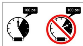
This tool is designed to operate within a range of pressure between 85 psi and 100 psi (or between 6 bar and 7 bar). Connect this tool to a pressure controllable device so that you can work under fixed pressure. When operating this tool, never use it under pressure of 100 psi (or 7 bar) and over.
