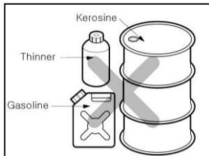
Never operate this tool near inflammables (such as thinner and gasoline). Combustible gas from such materials can be sucked into a compressor and compressed together with air, possibly resulting in explosion.
