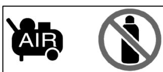
As this tool is designed and manufactured to operate using air pressure that is generated by an air compressor authorized by an safety certification authority, you cannot use any kind of gas—combustible gases such as oxygen and acetylene—except this. Otherwise, it may not only cause mechanical trouble but also malfunction or explosion, resulting in infliction of fatal injury on a user or those around him or her.
