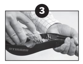
Place cap reel in basket. Insert lead cap under staples and feed through. Depress trigger to advance caps.
