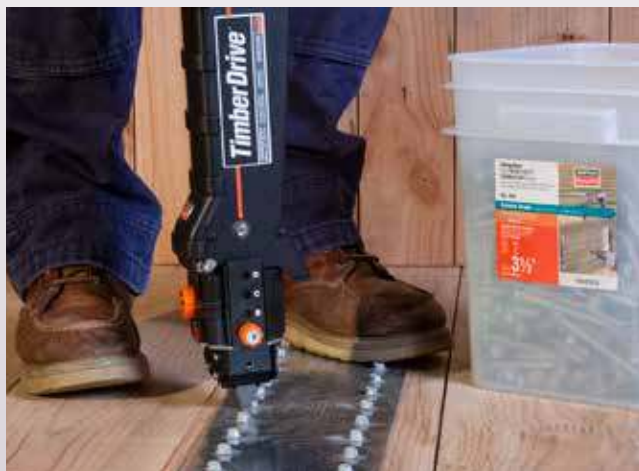
Precision-placement nosepiece for steel-to-wood fastening.
