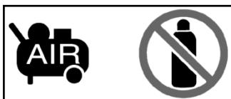
As this tool is designed and manufactured to operate using air pressure that is generated by an air compressor authorized by an safety certification authority, you cannot use any kind of gas—combustible gases such as oxygen and acetylene—except this. Otherwise, it may not only cause mechanical trouble but also malfunction or explosion, resulting in infliction of fatal injury on a user or those around him or her.
